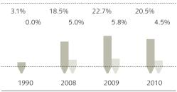
The alternative fuel ratio fell between 2009 and 2010, because we could only use a smaller amount of alternative fuels despite the rise in clinker production.
